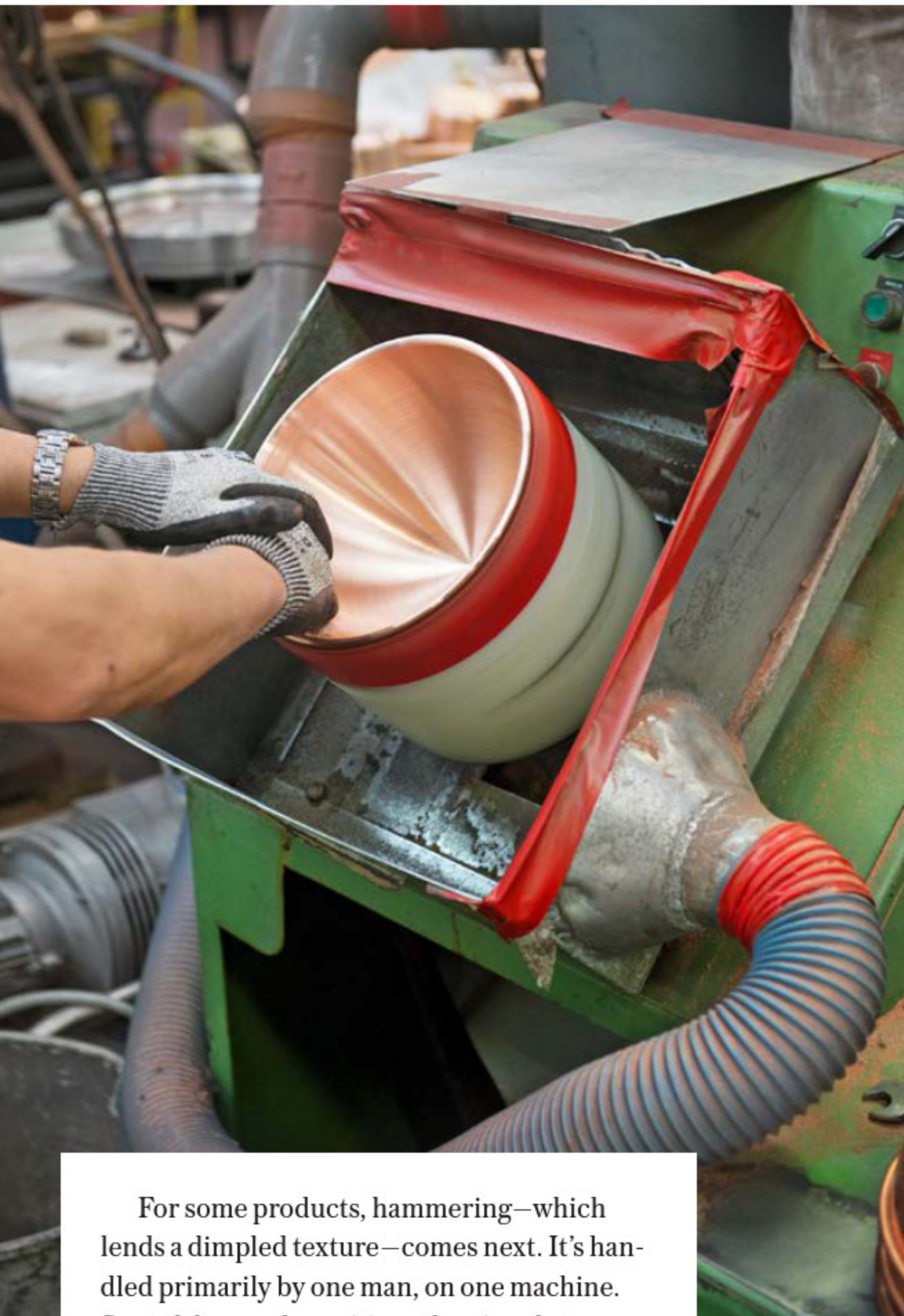
Among the final steps in the creation of Mauviel cookware are “shelving” and “spinning,” left, and a chemical-bath color treatment, right.
